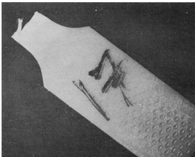
Fig. 15. Evidence of ductile behavior (tearing) in an 80% excess amine MDA-cured rubber-modified sample.
